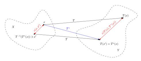
Figure 3.13. Forward errors (right) and backward errors (left).
