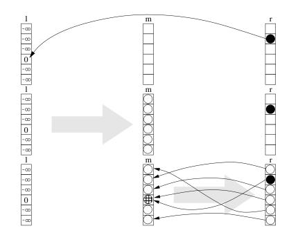
Figure 3.9. Finding the middle of an optimal path. A method to reconstruct the optimal path in short time, without storing the entire table.
