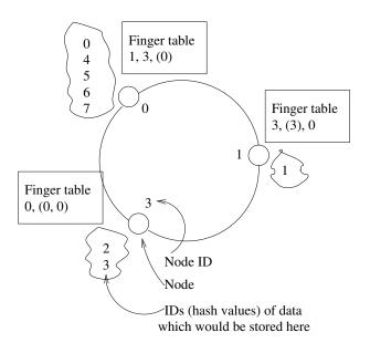
Figure 3.6. A Chord ring with 3 nodes with IDs 0, 1, and 3. Data is always stored in the node whose ID follows the data's ID, and thus, data with ID 0, 4, 5, 6, 7 is stored in node with ID 0, and data with ID 2 or 3 is stored in node with ID 3.
